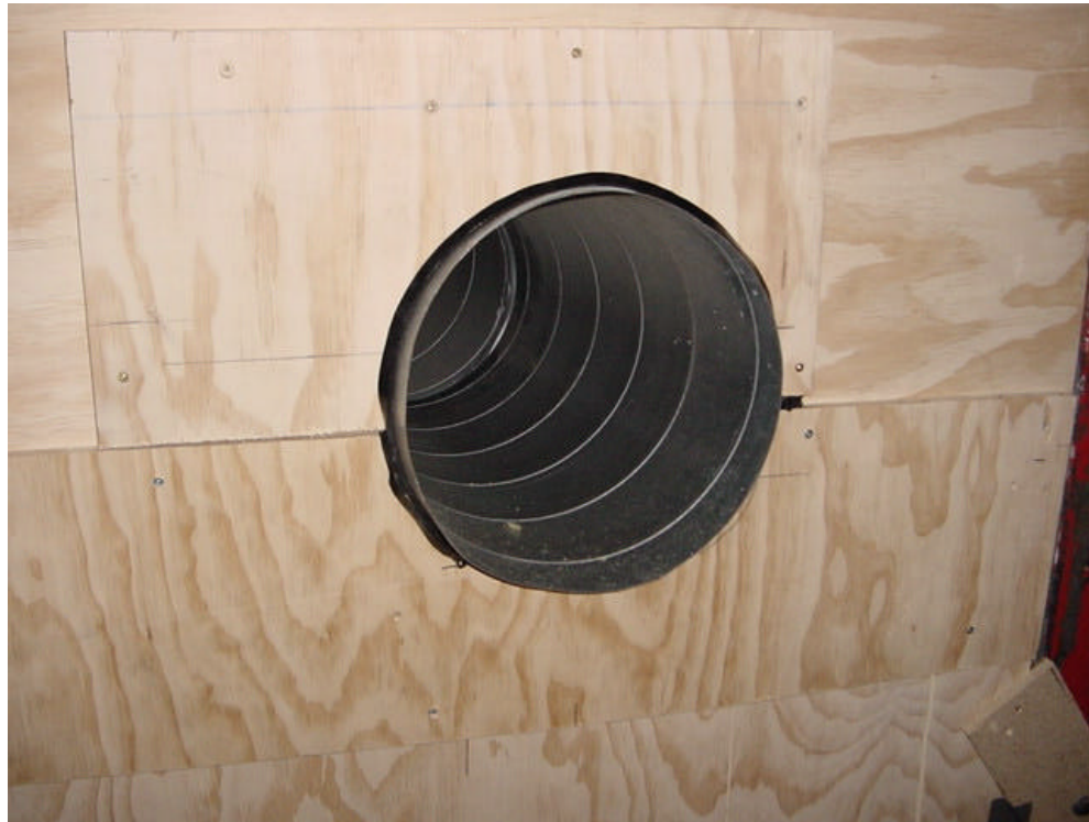
Photo B3: Outlet to Reverberation Test Chamber
