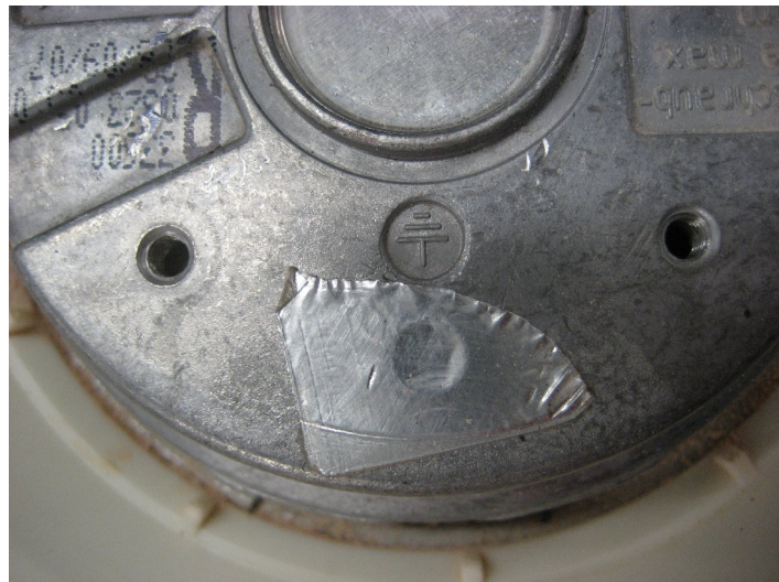
Figure 5 – Exposed screw hole sealed with aluminium tape before test
