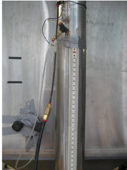
Figure 3 – Test setup showing manometer and flow meter
